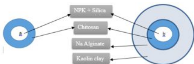
Schematic diagram of different coatings in CRF beads.
